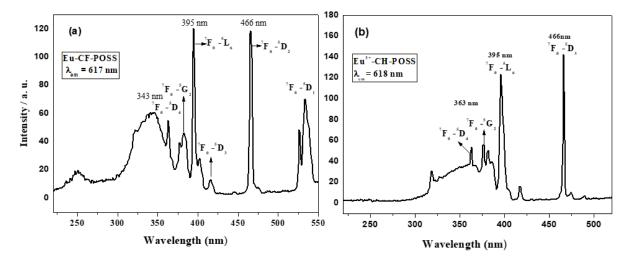
Fig. 5. Excitation spectra of (a) Eu<sup>3+</sup>-CF-POSS; (b) Eu<sup>3+</sup>-CH-POSS.
