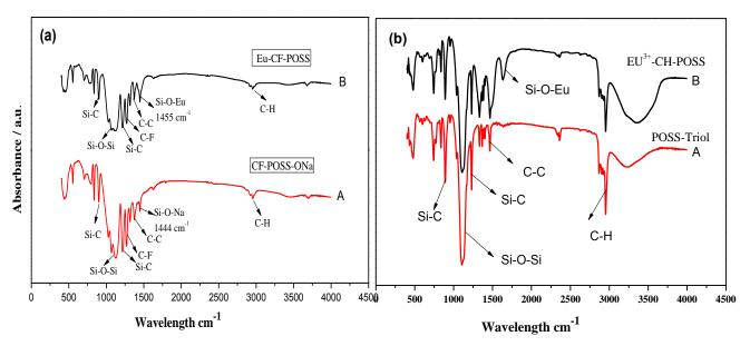
**Fig. 2.** FT-IR spectra of **(a)** europium free (7F-T<sub>7</sub>-(ONa)<sub>3</sub> (A) and Eu<sup>3+</sup>-CH-POSS (B); **(b)** POSS triol (A) and Eu<sup>3+</sup>-CH-POSS (B).
