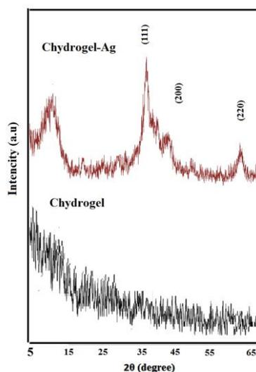
**Fig. 2.** XRD pattern of Chydrogel and Chydrogel–Ag nanocomposites.
