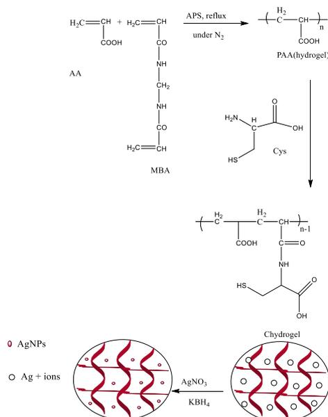
**Scheme.1.** Synthetic scheme for the preparation of the Hydrogel-Ag NPs composite.
