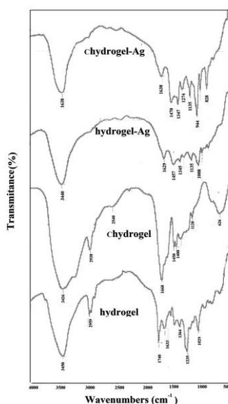
**Fig. 3.** FT-IR spectra of hydrogel, Chydrogel, hydrogel–Ag and Chydrogel–Ag nanocomposites.
