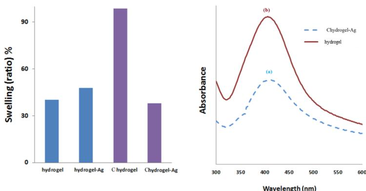
**Fig. 1.** A: Swelling behavior of pure hydrogel, Chydrogel, Ag-hydrogel and Ag-Chydrogel nanocomposites and B: UV-Vis spectra analysis of hydrogel–Ag and Chydrogel–Ag nanocomposites.
