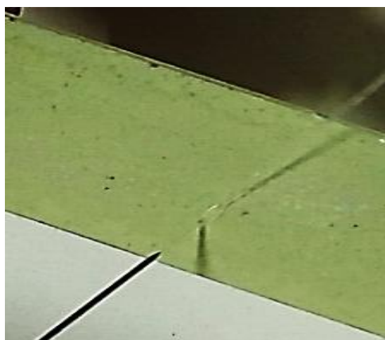
Figure 5. water jet impact of WO 3 nanoparticles coated polysilicon surface
