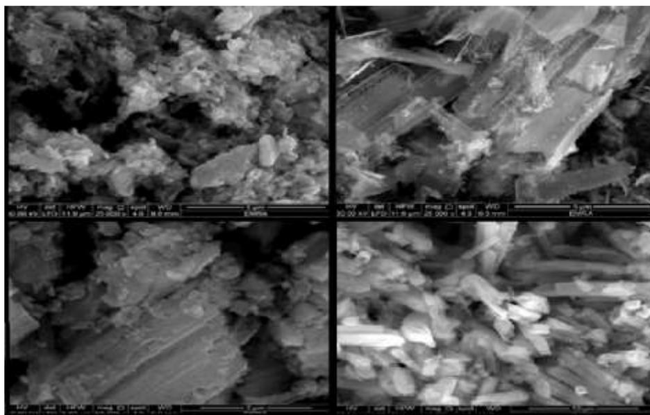
**Figure 5.** SEM images of TiO<sub>2</sub> nano powders calcined at 1000 °C prepared from a) methanol, b) isopropanol, and c) isobutyl alcohol
