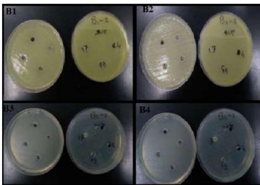
**Figure 6.** Effect of the different concentrations of of TiO<sub>2</sub> NPs (17= 800 µg/mL, 19= 200 µg/mL and 24=50 µg/mL) and sterilized distilled water (-ve= negative control) on B1) *Escherichia coli*, B2) *Klebsiella* sp, B3) *Staphylococcus aureus*, and B4) *Streptococcus* sp
