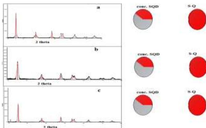
**Figure 2.** The XRD pattern, a) SQD conc., S-Q for  $TiO_2$  nanoparticles prepared, b) methanol, and c) isopropanol, isobutyl alcohol calcined at 400 °C
