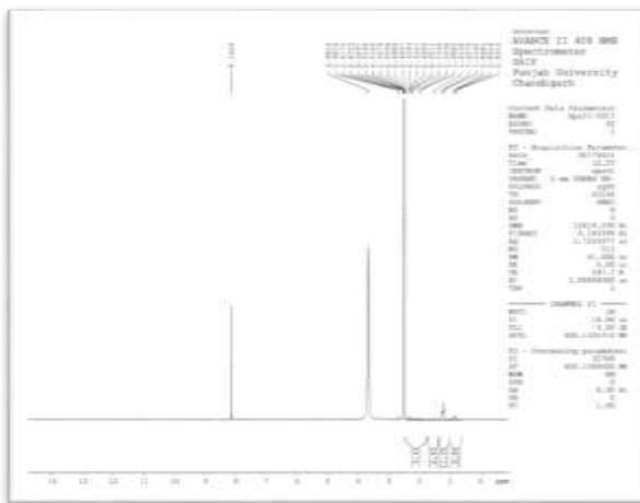
**Figure 4.** NMR spectra of isolated biopolymer P
