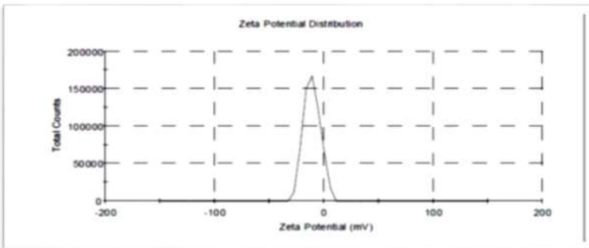
**Figure 2.** Zeta potential curve for nanosize olanzapine
