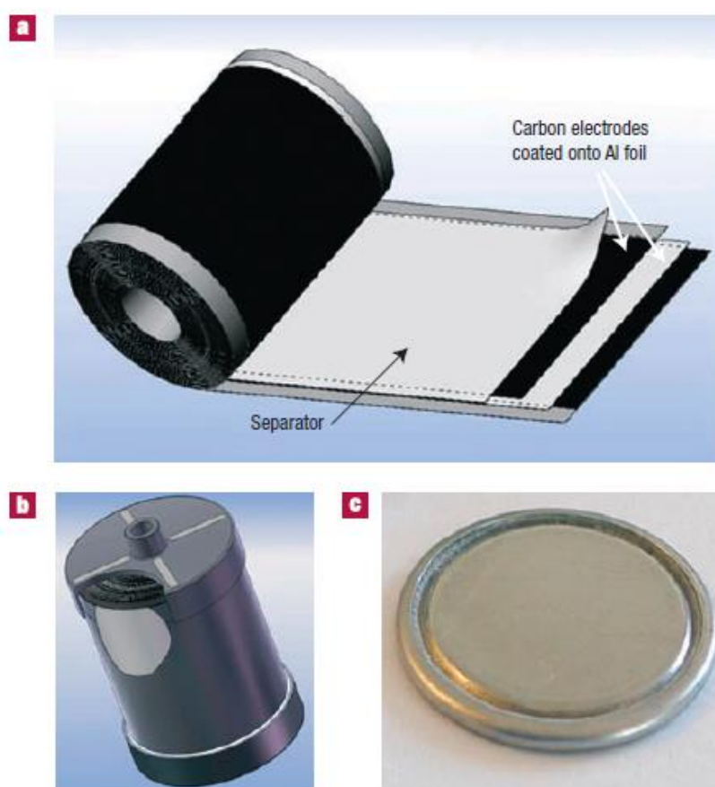
Fig.5 Electrochemical capacitors. a Schematic of a commercial spirally wound double layer capacitor. b , Assembled device weighing 500 g and rated for 2,600 F (Photo courtesy of Batscap, Groupe Bolloré, France.) c , a small button cell, which is just 1.6 mm in height and stores 5 F. (Photo courtesy of Y-Carbon, US.) Both devices operate at 2.7 V [17].
